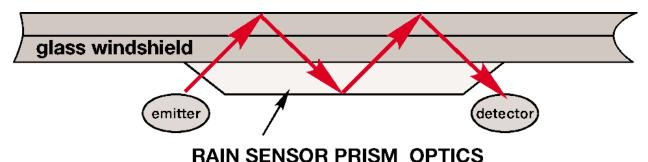
The density of water is closer to that of glass than air. When rain starts to accumulate in the sensor monitoring area, it causes part of the infra red beam to extend past the outside surface of the glass and into the rain drop. When this occurs, the beam is refracted and only part of the beam returns to the detector diode.
